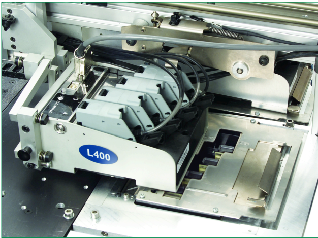
Bulk Ink print head entering Maintenance Station
